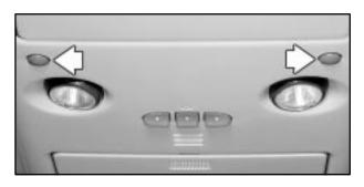
Your vehicle has front reading lamps located in the overhead console. Press the round button located next to the lamp to turn the lamp on. The lamps can be adjusted to point in the direction you want them to go.
